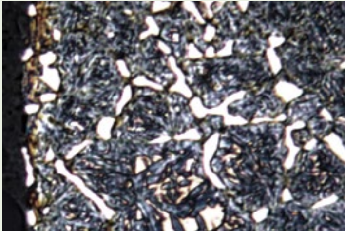
Figure 1: Microstructure of carburized case where a high carbon potential resulted in excessive carbide formation.
