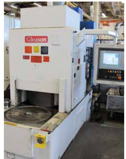
Figure 1. Example of a modern quenching machine. [Photograph courtesy of The Gleason Works, Rochester, NY].
