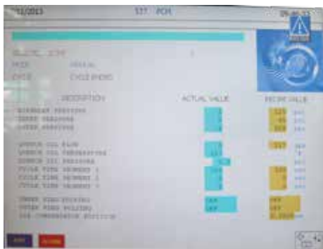
Figure 2. Control screen showing the various parameters that may be adjusted over the course of a typical quenching cycle. (Photograph courtesy of The Gleason Works, Rochester, NY).
