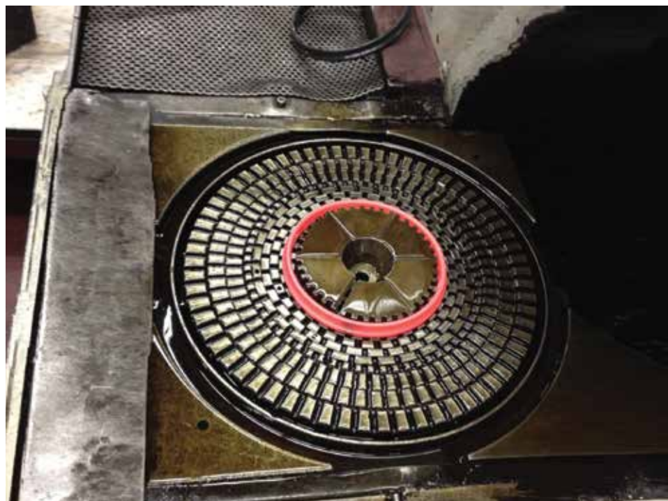
Figure 3. Hot bearing race positioned on the lower die assembly of a quenching machine just before it is retracted into the machine for quenching. Note the segmented die tooling and individual slotted rings. The slotted rings may be independently adjusted to control the flow of oil over the part being quenched. (Photograph courtesy of The Gleason Works, Rochester, NY).
