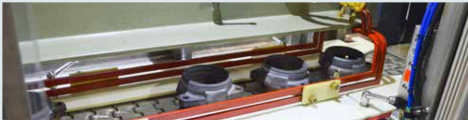
Image 2: Channel coil uses a separate lower-frequency power supply to heat multiple parts at the same time while parts are moved forward on a conveyor.
