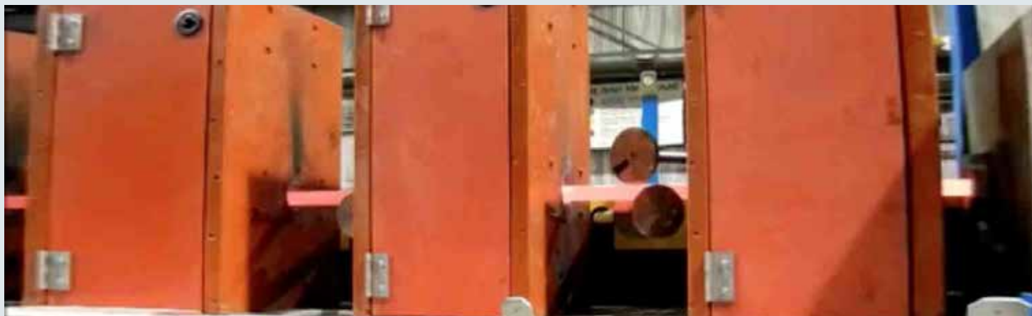
Image 1: Solid bar is heated progressively using a series of induction coils to austenitizing temperature prior to quenching and tempering.
