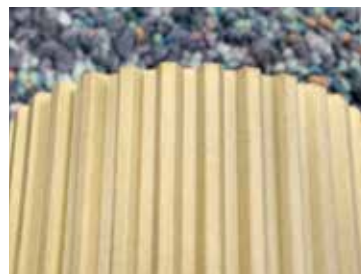
Figure 9: Gear shafts made of Ti-6Al-4V alloy after plasma nitriding at 730°C in pure nitrogen: Gold color is a characteristic of titanium nitride film formed during nitriding
