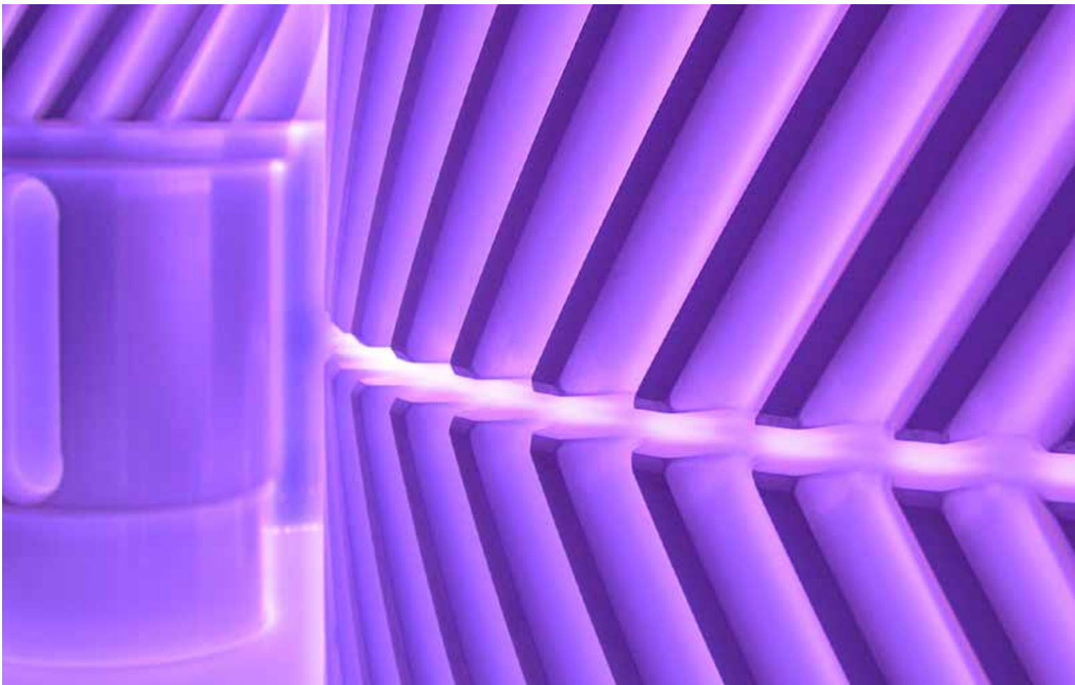
Figure 1: Large gear shafts during ion nitriding
