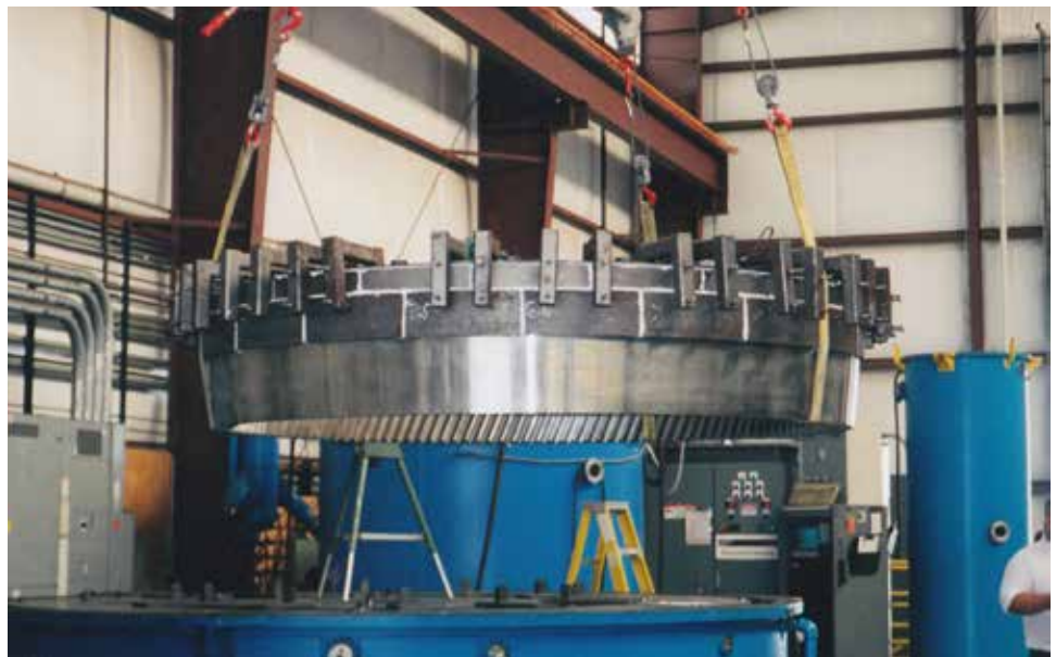
Figure 5: Plasma nitriding of the AISI 4340 alloy-steel gear used in the power industry. Mechanical masking/segmented fixturing covers a portion of the outside diameter of the gear to perform selective hardening.
