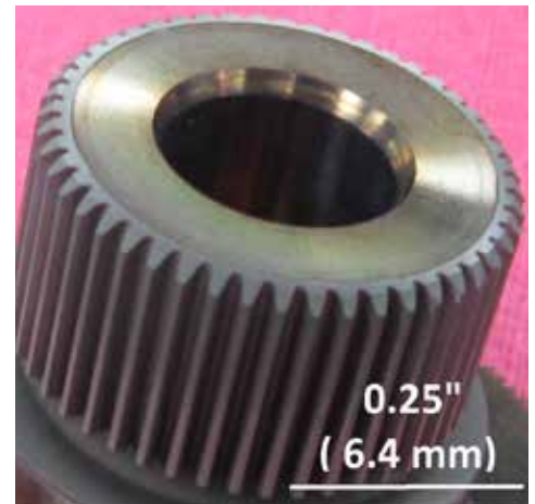
Figure 2: Small 15-5 PH steel gear for the aerospace application after plasma nitriding. Note nitrided teeth and all the other surfaces protected from the treatment by mechanical masking. The diametral pitch was 50.
