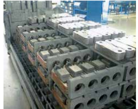
Fig 2: Load of Heat Exchangers for Brazing
