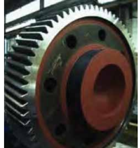
Figure 12: Example of a larger gear designed as a welded construction
