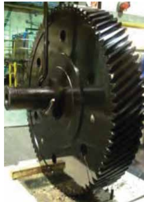
Figure 22: Example of different possible charging method (vertical charging)
