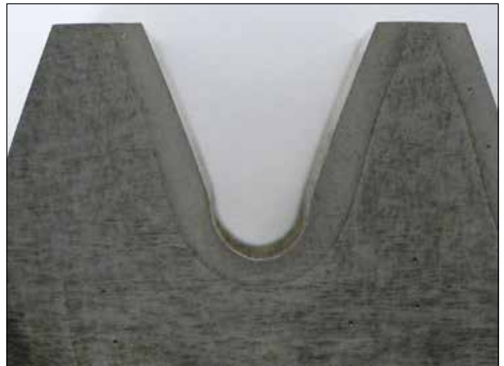
Figure 3b: Carefully positioned quench heads provide quenchant where needed to cool the tip and the flank to achieve the desired hardening pattern and minimize back tempering.
