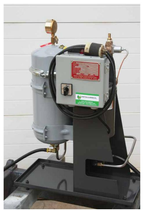
that pump to remotely look at all the pump operating parameters (is the pump running, oil temperature, oil level). You can access a small PLC on the pump from your plant Ethernet system. If it's plugged into the Ethernet IP network in your facility, you can access it from a smartphone."
