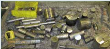
Figure 1: A wide assortment of shafts with splines, rounds, hex shapes, holes, flanges and each takes planning as to how to cut the work piece.
