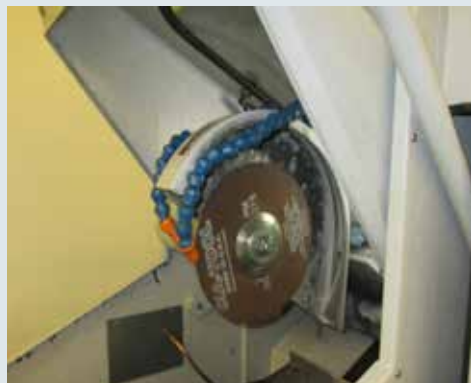
Figure 2 A & B: Two adjustable point of contact nozzles for cooling both sides of saw blade and work piece.
