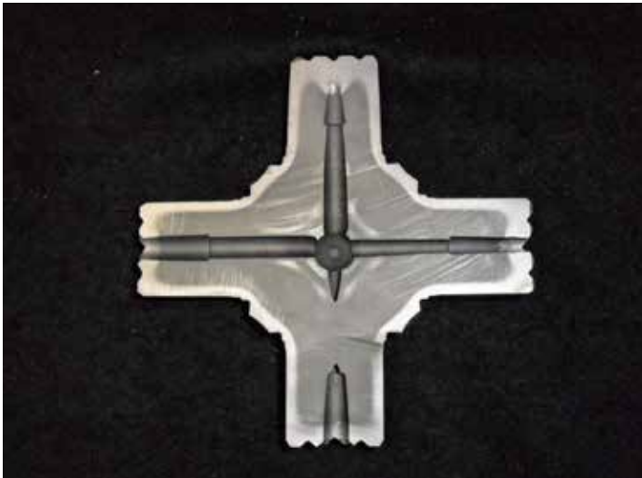
Figure 8: Induction hardened automotive journal cross. (Courtesy of ERS Engineering Corp.)
