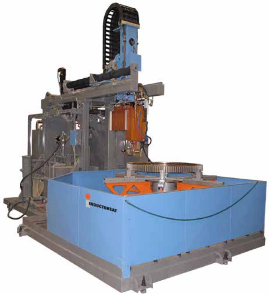
Figure 2: Induction gear hardening machine for a large bearing ring with teeth located on outside [Courtesy of Inductoheat Inc.]
