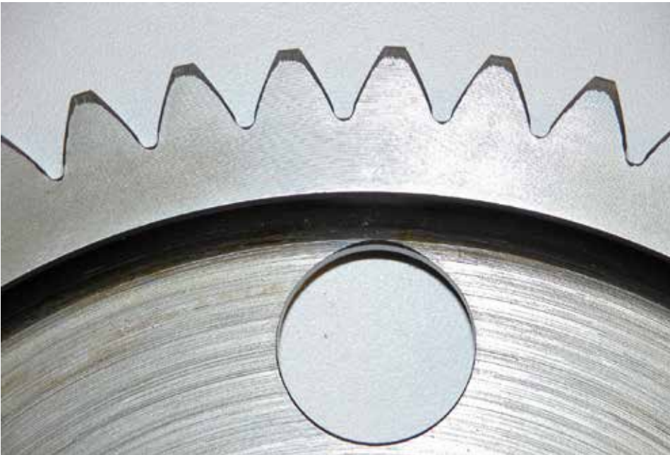
Figure 7: Improper hole placement.
