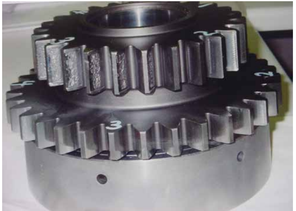
Figure 5: Inadequate hardness leading to gear failure.
