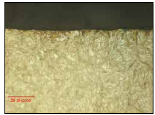
Fig. 6: No presence of intergranular oxidation after LPC process.
