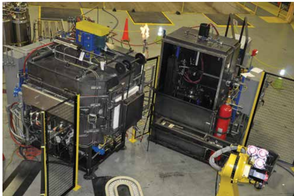
Figure 3: The custom-designed, fully-automated heat treatment and material handling system .
