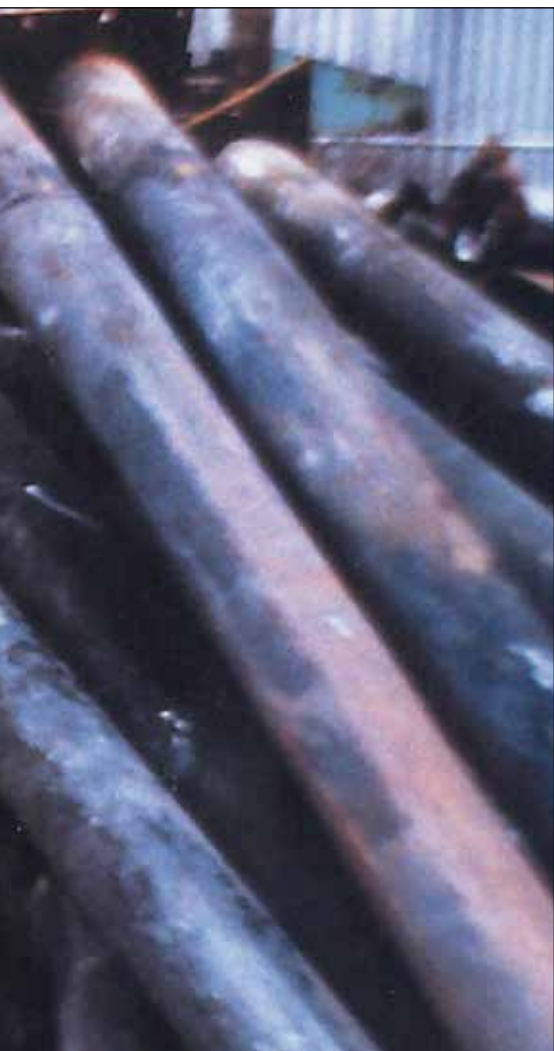
Fig 1: Expensive alloys can creep, distort, and rupture in a short time.
