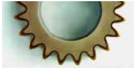
Fig 12: Precise, repeatable contour of complex geometries—a gear hardened by simultaneous-dual frequency induction heating.
