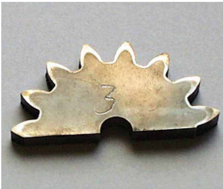
Fig 7: The end-result of single-frequency inductive hardening.
