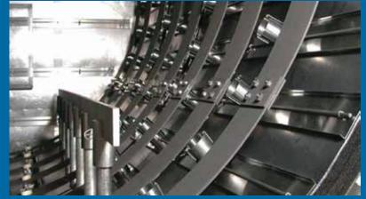
surface and internal contaminants on molten metal applications are volatized and removed. Heating is fast and efficient using radiant energy that heats only the product in the vacuum environment.
