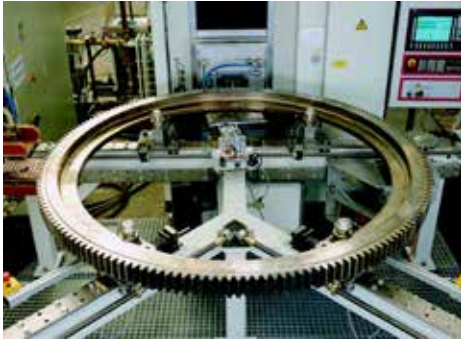
Figure 8: Typical Induction Heat Treated Gear. (Photograph Courtesy of EMA Induction Technology)
