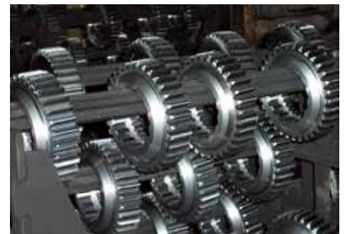
Figure 4: Typical Load of Truck Transmission Gears Processed in a Pusher Furnace.
