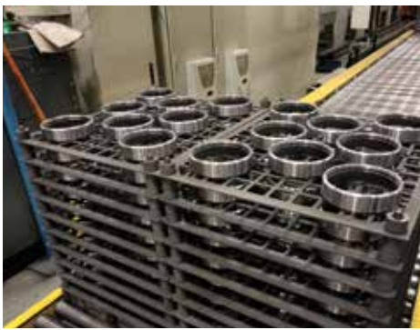
Figure 7: Typical Load of Gears for LPC Carburizing. (Photograph Courtesy of ALD Thermal Treatment)
