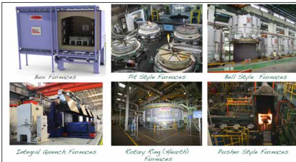
Figure 1: Typical Batch Style Furnaces.
