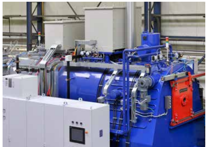
Figure 6: Typical Vacuum Hardening and Case Hardening Furnace. (Photograph Courtesy of SECO/WARWICK Corporation)
