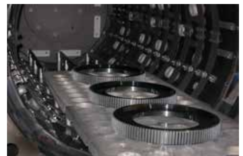
Figure 5: Vacuum Hardening and/or Carburizing of Gears. (Photograph Courtesy of Solar Manufacturing)
