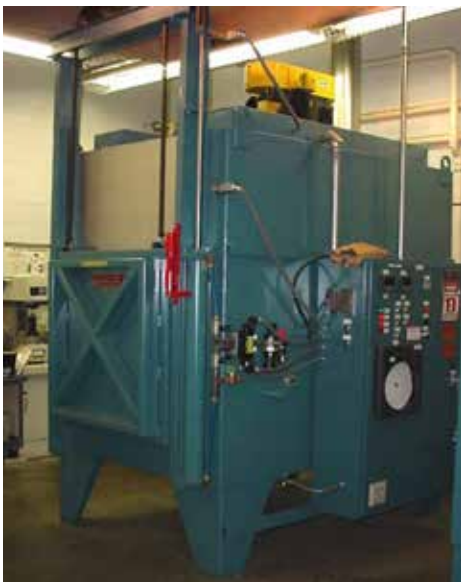
Figure 9: Typical Ovens Used for Tempering Gears. (Photograph Courtesy of Wisconsin Oven Corporation)
