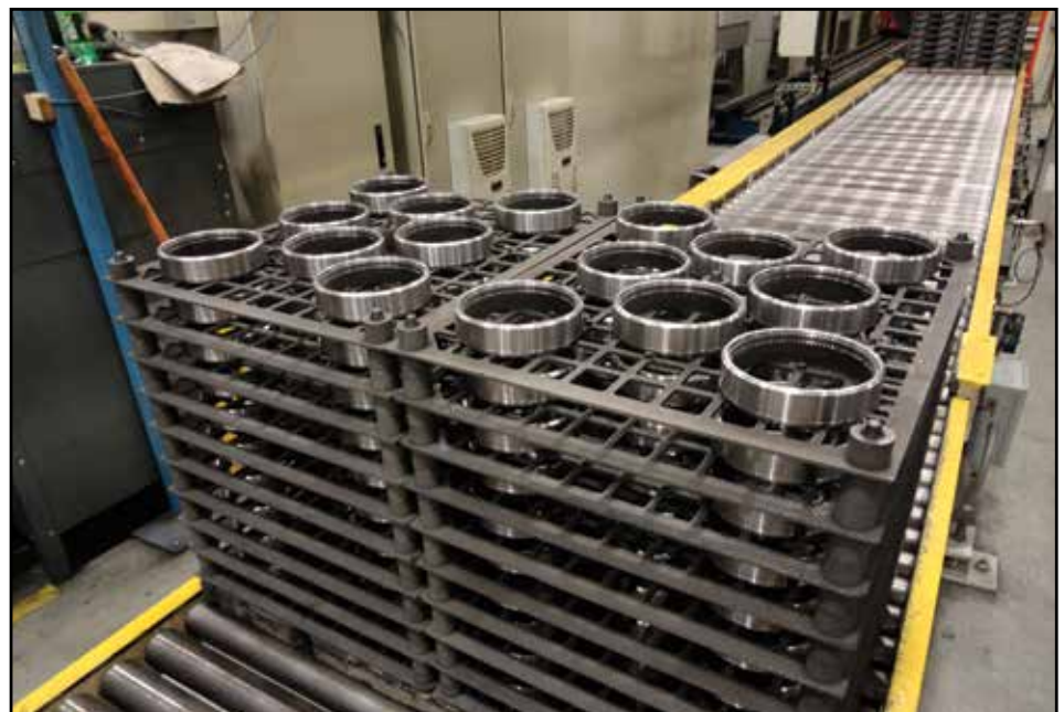
Figure 3: Present Day Commercial Heat Treat Load, February 2012. Gears Carburized at 930°C (1700°F), 14.5 mbar (11 torr), Acetylene [C 2 H 2 ]. (Photograph Courtesy of ALD Thermal Treatment)
