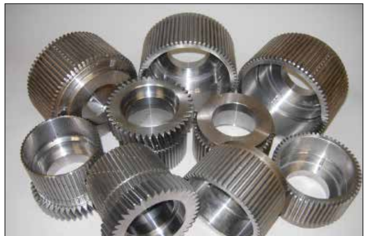
Figure 10: Vacuum Carburizing of Highly Distorted Prone Gearing.
