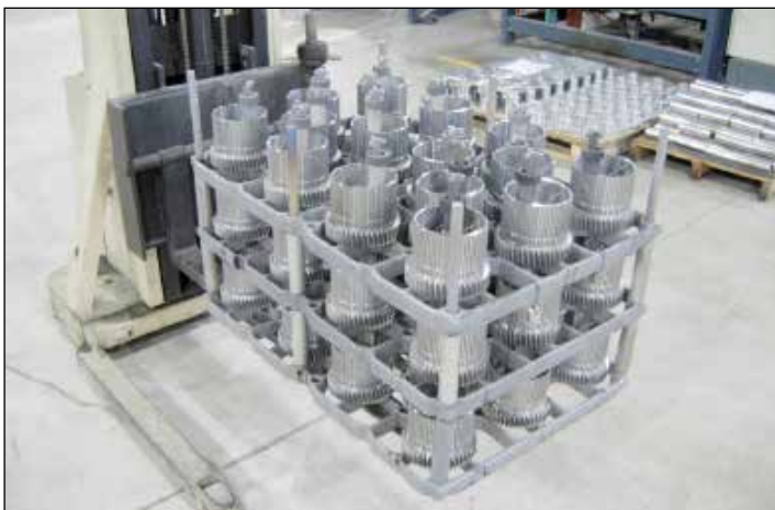
Figure 9: Typical Furnace Load, 385 kg (850 lbs.).
