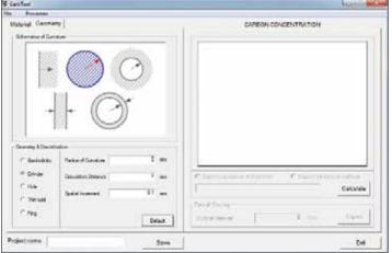
Users input data, including the carburization temperature, time, and carbon potential or flux, and by using the simulation software, the heat treater can determine the carbon concentration below the surface to plot case depth according to a user-defined value.
