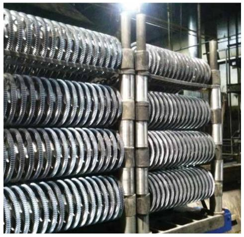
Figure 2: Carburizing hanging fixture for heavy truck gears.
