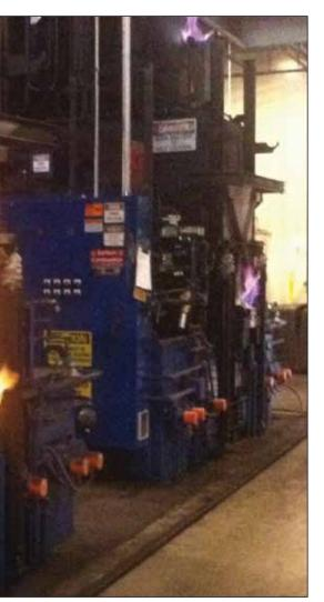
Batch Integral Quenching Furnace used for Carburizing Gears at Bluewater Thermal Solutions – Greensburg, IN.
