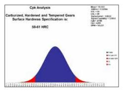
Figure 1: CPK Analysis using 59-61 HRC Specification Range.
