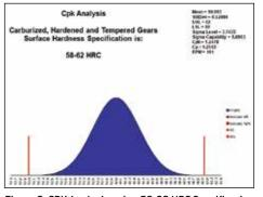
Figure 3: CPK Analysis using 58-62 HRC Specification Range.
