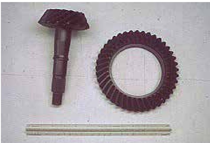
Figure 7: A rear differential hypoid gear and pinion set. ADI replaced carburized and hardened steel, eliminated the need for a press quench, increased machine tool life, reduced gearbox noise, increased the torsional ultimate strength, decreased scoring, and reduced the overall cost of the gear set. [1]
