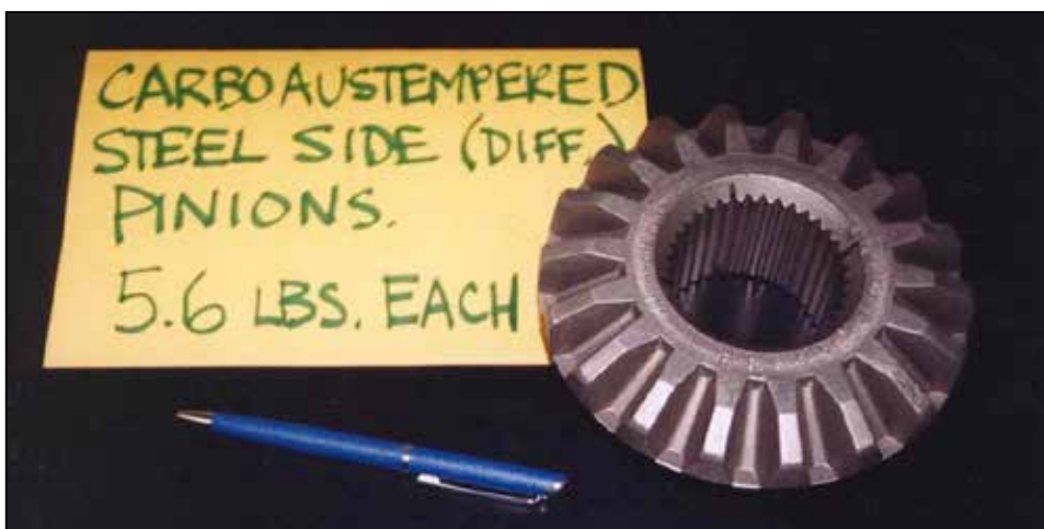
Figure 12: A Carbo-Austempered™ differential side pinion for a severe-duty off-highway truck. Courtesy of Dana Corporation.
