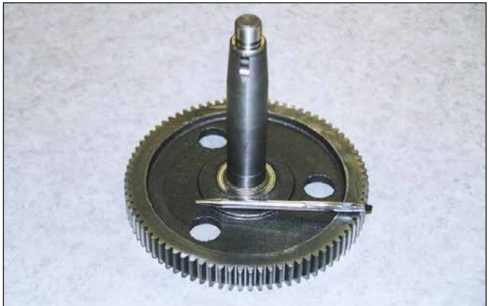
Figure 9: This gear and axle is in the final drive of a commercial riding mower. ADI replaced a three piece carburized and hardened steel assembly. There are no known service failures of this part Courtesy of Farrar Corporation.
