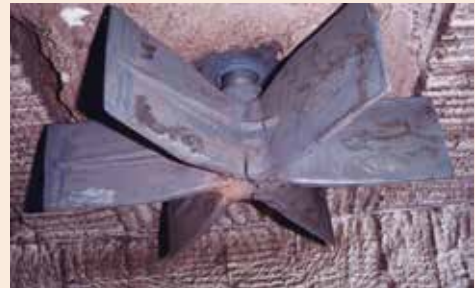
Figure 5: Thermal fatigue cracks in roof fan
