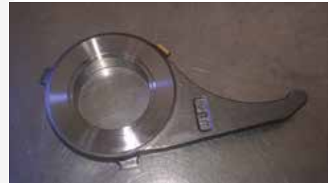
Figure 3: Lever made of 8620H material
