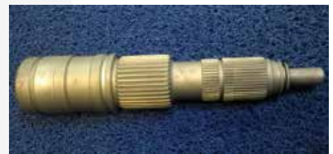
Figure 4: Shafts made of 28MnCrB7-2 material
