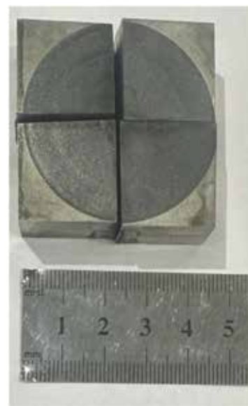
Figure 2: Samples after mechanical treatment prepared for electrolytic-plasma nitriding.
