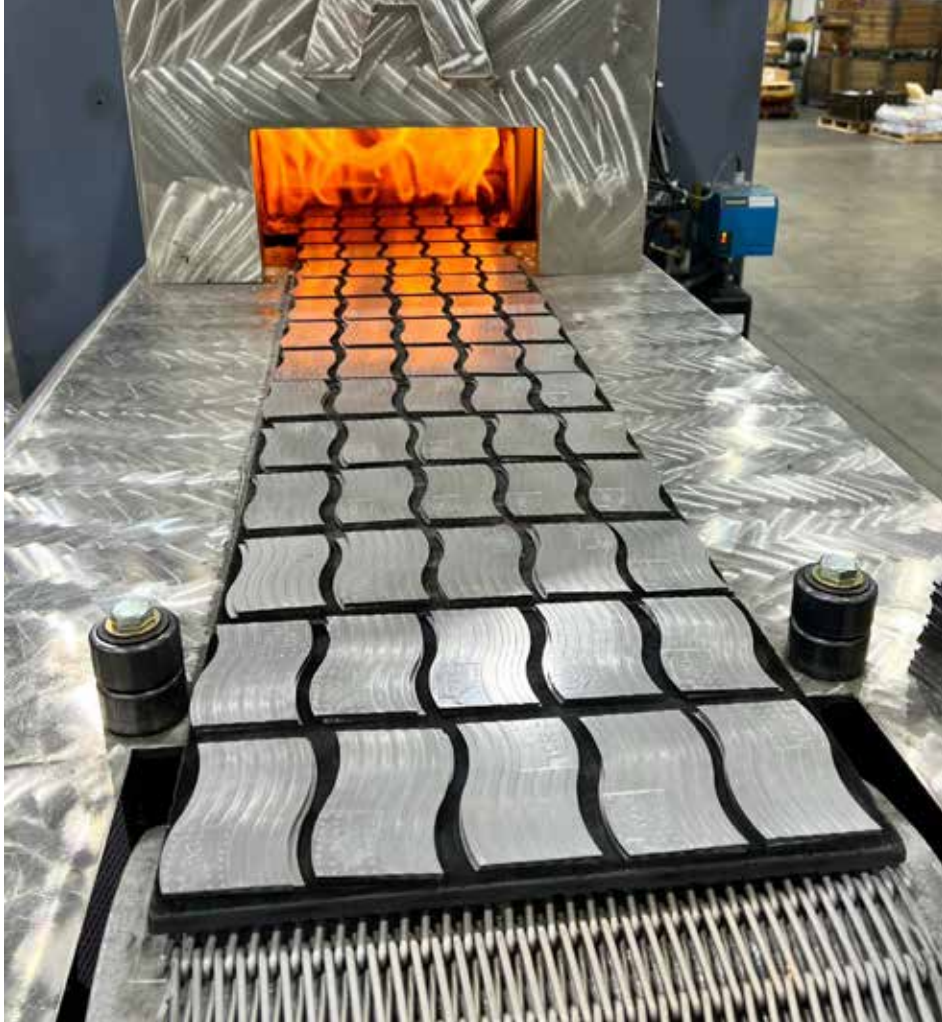
Parts entering Abbott Furnace's seven-zone continuous belt sintering furnace at Metco Industries in St. Marys, PA. (Courtesy: Abbott Furnace Company)
