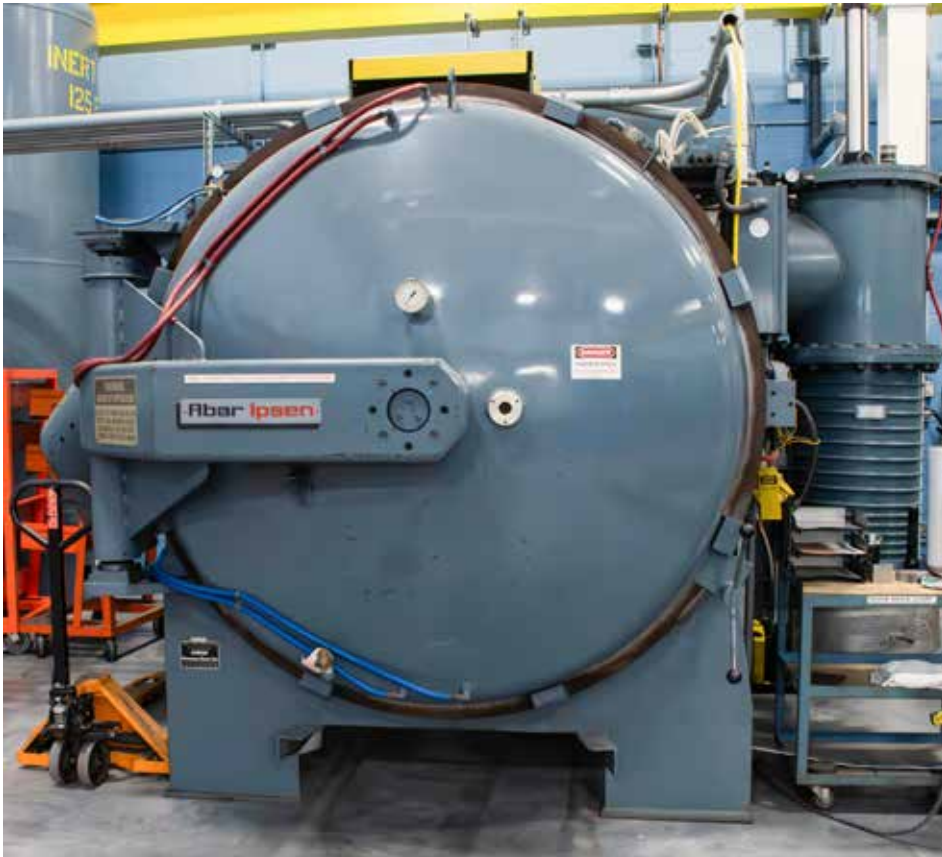
Urschel Laboratories, Inc. has purchased an Ipsen MetalMaster® HR 54x48 2-bar vacuum furnace to replace a MetalMaster furnace from 1986 that has been in continuous use. (Courtesy: Ipsen USA)
