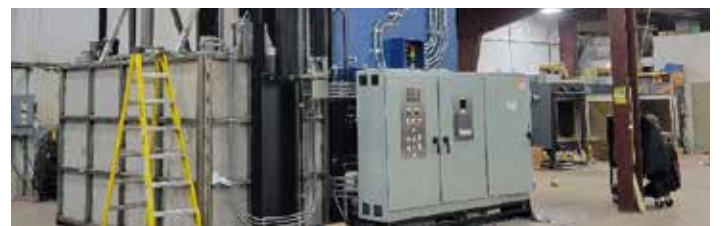
A horizontal aluminum quench furnace sold by W.H. Kay. (Courtesy: W.H. Kay)
