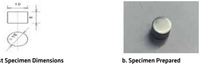
Figure 1: Microhardness and SEM analysis specimen as per ASTM E384 standards [20].
