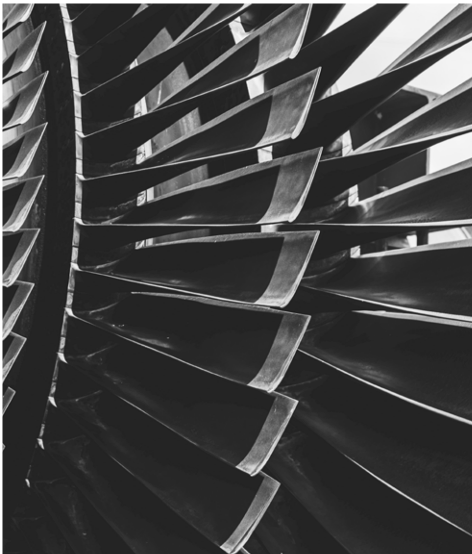
Nickel-based superalloys are the largest class of superalloys due to excellent high-temperature strength and oxidation resistance. They are most often used in the hottest sections of gas turbines, and include the turbine blades, vanes, and hubs. (Courtesy: Shutterstock)
