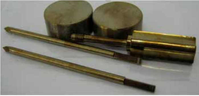
Figure 6: Sample of stainless-steel parts contaminated by gas from the rusty inside of a buffer tank. (Courtesy: Ipsen)
