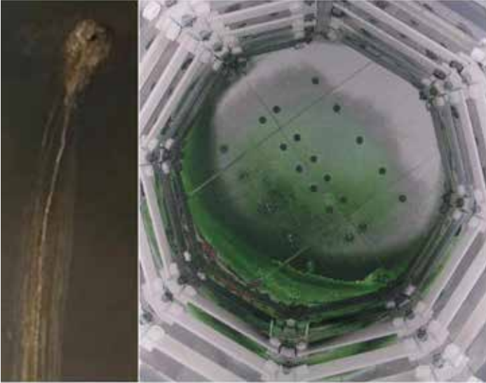
Figure 7: Left – internal vessel weld. Right – Graphite hot zone exhibits significant water damage caused by a heat exchanger leak, resulting in prominent forest green discoloration. (Courtesy: Ipsen)
