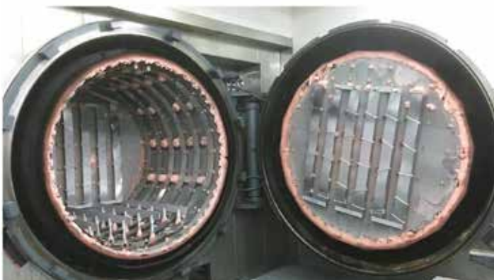
Figure 9: Discoloration caused by copper material during the brazing process. (Courtesy: Ipsen)
