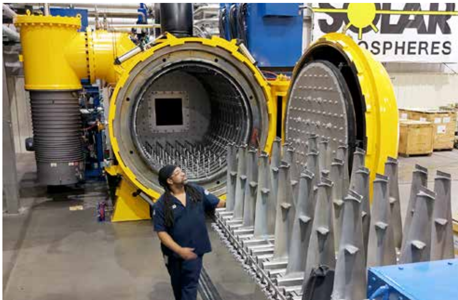
Solar Atmospheres' new 10-bar vacuum furnace at its Greenville, South Carolina, facility will provide another regional option for high-pressure quenching of large components and workloads. (Courtesy: Solar Atmospheres)
