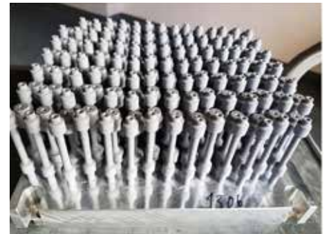
Figure 8: Print job with 103 static and 103 fatigue test specimens. The two types of samples were arranged in pairs to investigate local dependencies in print quality within the build space.
