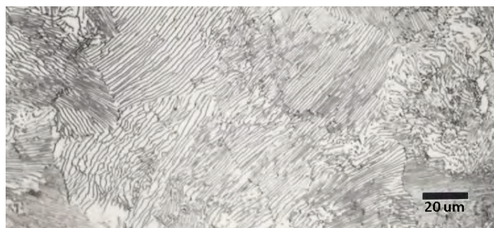
Figure 1: Microstructure of a hot-rolled SAE 1080 steel, slow cooled to form 100 percent pearlite. Etched in picral.
