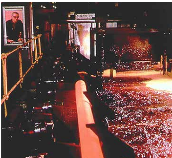
Figure 24: Quenching of critical alloy steel tubing for oil industry in 20% ACR polymer.
