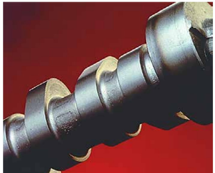
Figure 12: Induction-hardened camshaft quenched with PEOX polymer quenchant showing freedom from sticky deposits.
