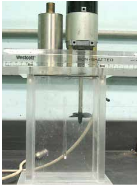
Figure 2: Tensi apparatus for testing polymer quenchants, as described in ASTM D6482 [1].
