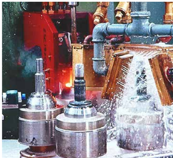
Figure 8: Induction hardening of an automotive constant velocity joint using a PAG at 7%.
