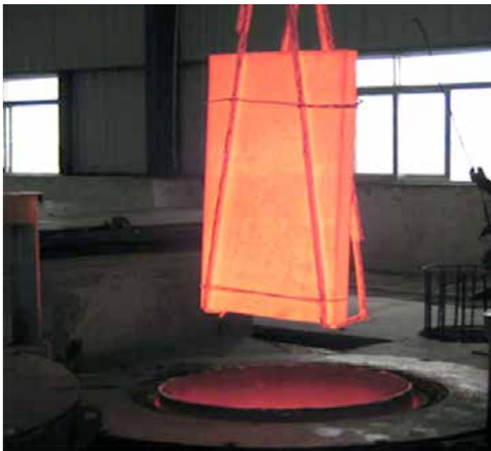
Figure 18: Large AISI 420 stainless steel weighing 500 kg quenched into 18 percent PVP with resulting hardness of HRC 54-56.
