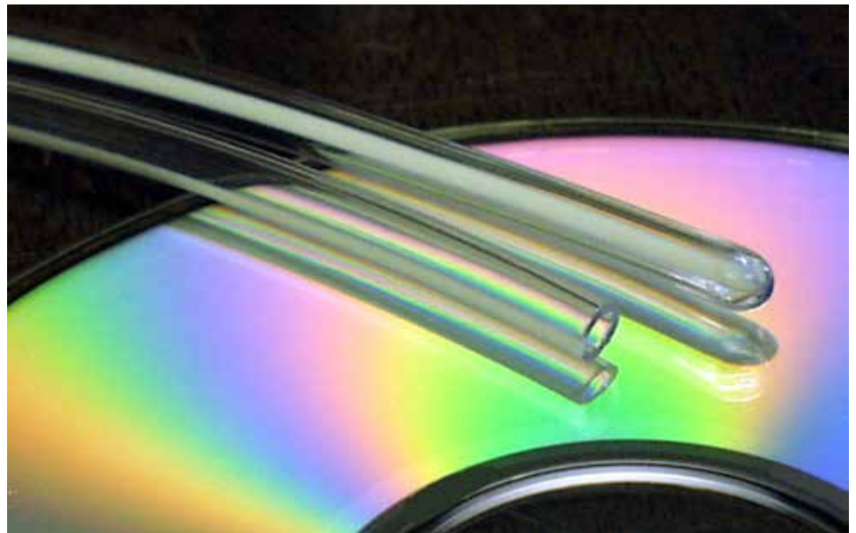
Forming the tips of small catheters is commonly done with induction heating. (Courtesy: Ambrell)
