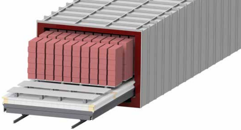
RATH developed lightweight lining for a tunnel kiln car, which now absorbs very little process heat. (Courtesy: RATH)
