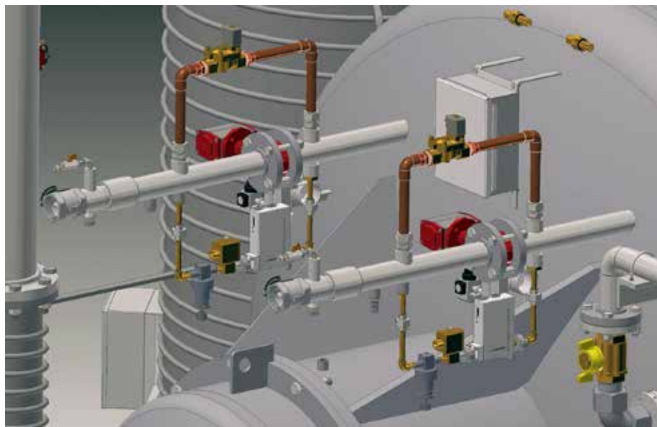
A furnace design that includes two ports for partial pressure gas, regulated by mass flow sensors.
