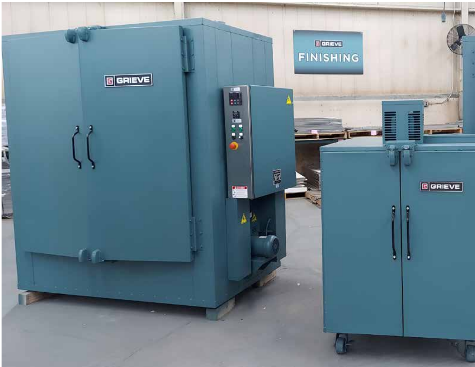
Finishing ovens. (Courtesy: The Grieve Corporation)
