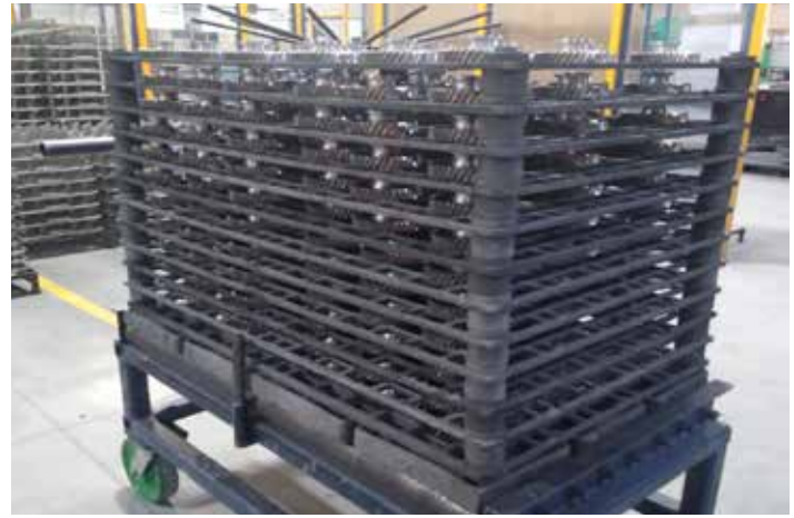
Figure 6: Load of sliding gears (CFC fixture consisting of 12 layers).
