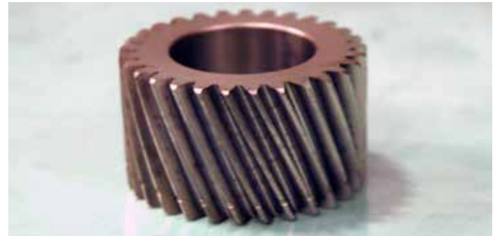
Figure 15: Final-drive pinion planetary gear (diameter = 31 mm, 24 teeth).
