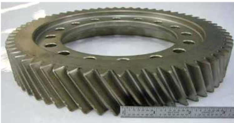
Figure 13: Final drive ring gear and production load consisting of nine layers.
