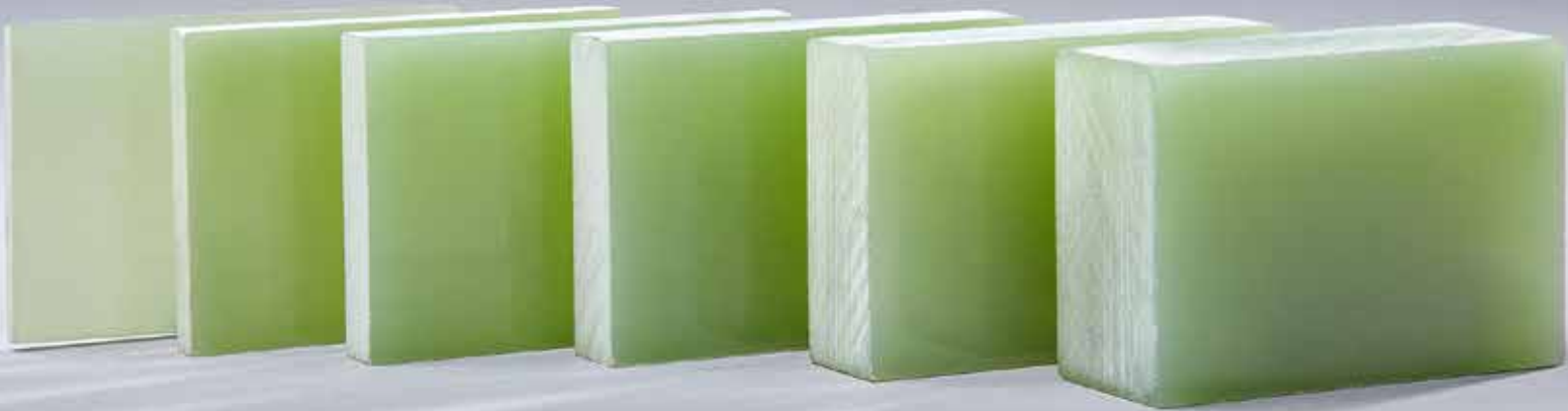
A variety of G10 laminated composites displaying the differing thicknesses. (Courtesy: Current Composites)
