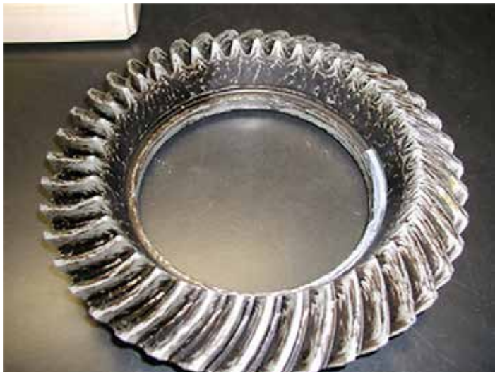
Figure 1: Typical staining from oxidation.
