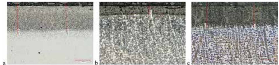
Figure 4: Microstructure of nitrided layer on substrate surfaced with materials: a) DO*15 Fe-Cr-Mo-W, b) DO*04, Fe-Cr-Co-Mo, c) DO*341, C-Cr-Ni-Mo.
