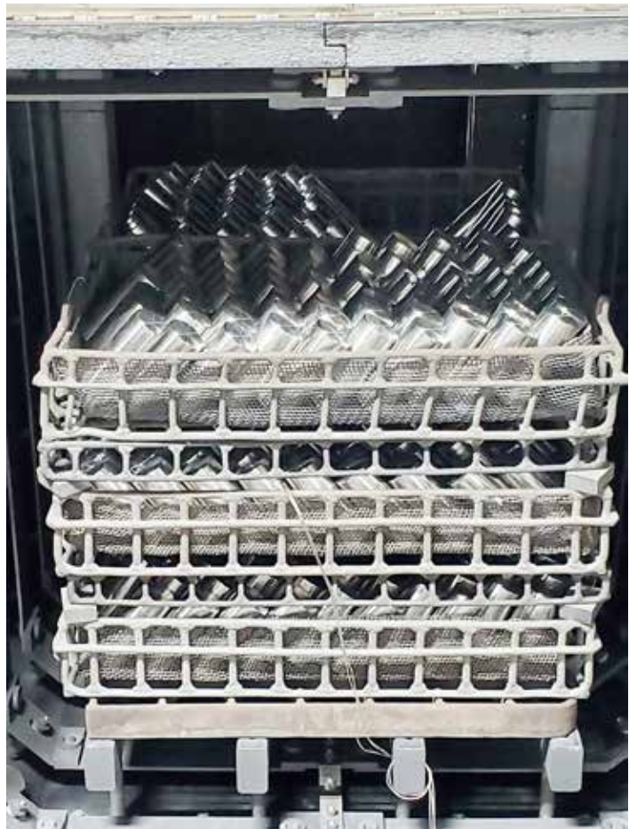
Figure 3: Bright, clean 4340 fittings post-oil quench.
