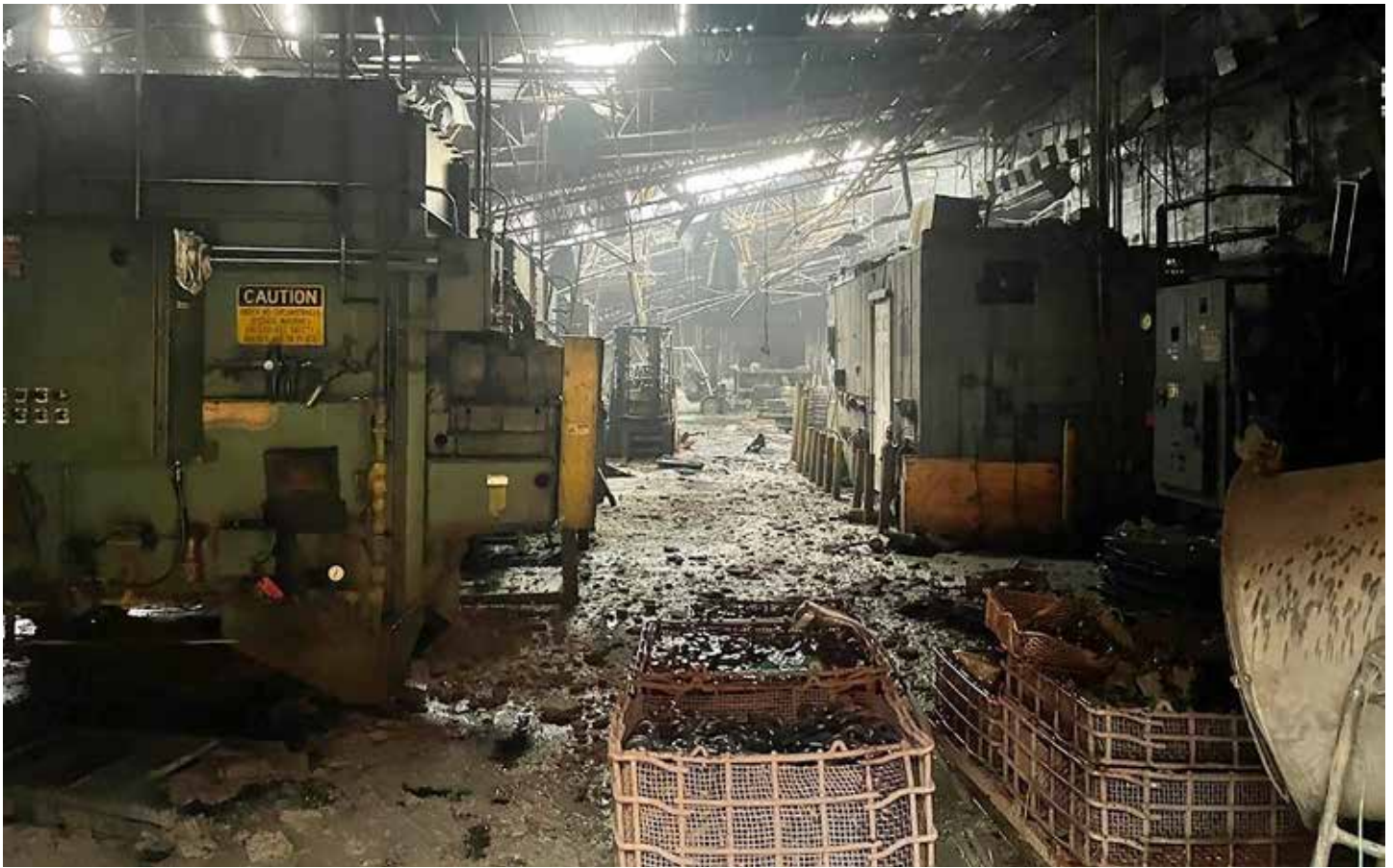
Figure 5: Catastrophic oil quench fire.
