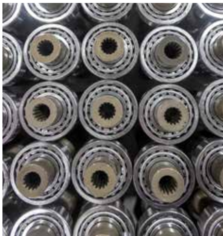
Kinematics' latest generation slew drive designed specifically for the challenges of solar tracking uses a grease free dry bearing design for increased holding torque and lower maintenance. (Courtesy: Kinematics)
