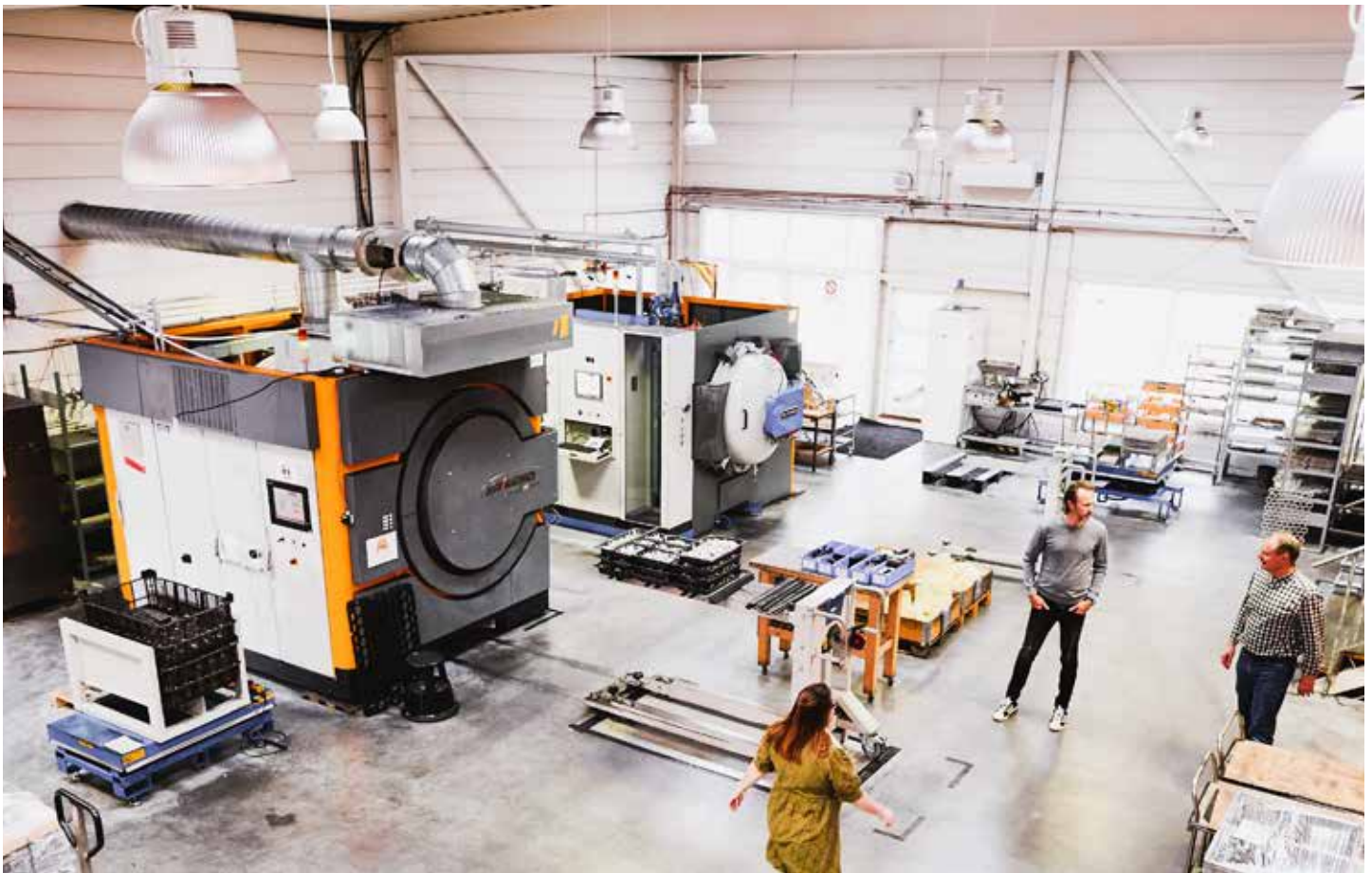
Expanite's innovative process is a gas-based diffusion technology that removes the oxide layer from the stainless steel. (Courtesy: Expanite)
