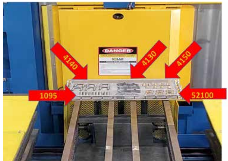
Figure 4: Various materials, similar thickness, processed together.
