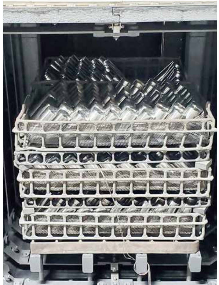
Figure 3: Bright, clean 4340 fittings post-oil quench.
