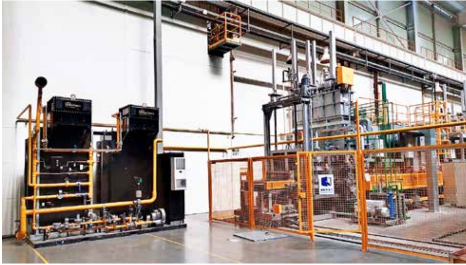
EndoFlex from UPC-Marathon offers several benefits, including precise control of production media to the carburizing and hardening environments, leading to higher quality gear production with improved longevity and performance. (Courtesy: Nitrex)
