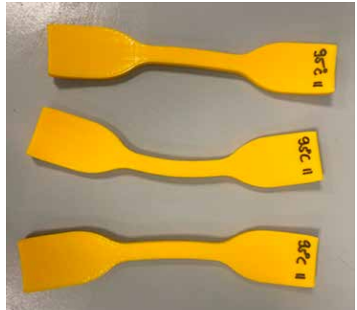
Figure 3: Deformed specimens after heat treatment.
