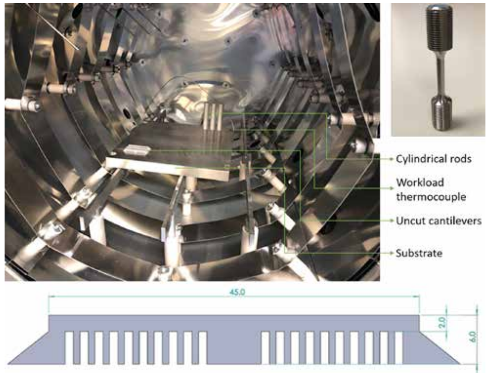
Figure 1: Ti6Al4V substrate with unmachined tensile rods and cantilevers inside the vacuum chamber. A typical machined tensile specimen is shown at the top right, and the cantilever specimen dimensions are at the bottom.
