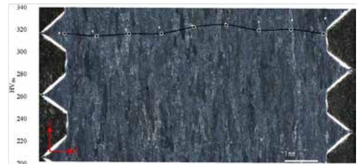
Figure 11: Vertical (XZ plane) cross-section and microhardness across the threaded section of a New-cycle tensile specimen.
