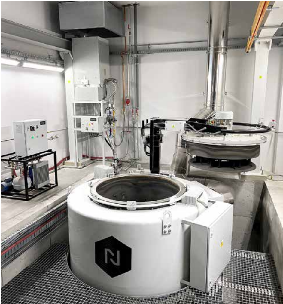
Extral Sp. z o.o. ordered a Nitrex nitriding system featuring the exclusive Nitreg® technology to nitride H11 and H13 extrusion dies of various sizes. (Courtesy: Nitrex)
