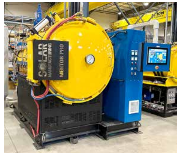
The Solar Manufacturing Mentor ® Pro Model HFL-3036-2IQ vacuum furnace features a molybdenum shielded hot zone measuring 18" wide x 18" high x 36" deep, capable of operating temperatures up to 2,400°F. (Courtesy: Solar Manufacturing)
