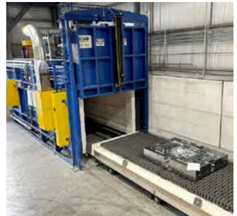
Solar Atmospheres of Western PA's newly installed car bottom air furnace is a benefit to customers and for production as it can be used for heavy parts as well as long components. (Courtesy: Solar Atmospheres of Western PA)
