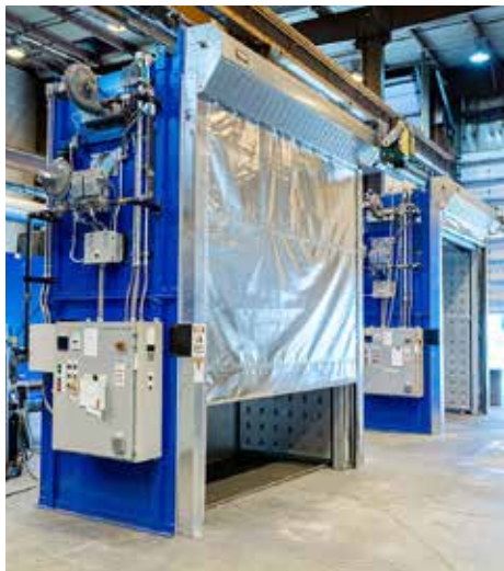
The Wisconsin Oven batch ovens have a maximum operating temperature of 350°F and work chamber dimensions of 9' wide x 4'6" long x 10'6" high. (Courtesy: Wisconsin Oven)
